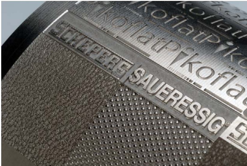
Figure 1: 3D surface of a leather and calotte embossing tool structured with picosecond lasers (Photo: Schepers GmbH & Co KG, Vreden, Fraunhofer Institute for Laser Technology ILT, Aachen)
